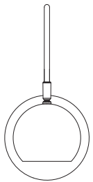
DHA05 one 3000K, 80CRI, 6.5 Watt, 600 Lumen LED Backplate: 5" diameter
